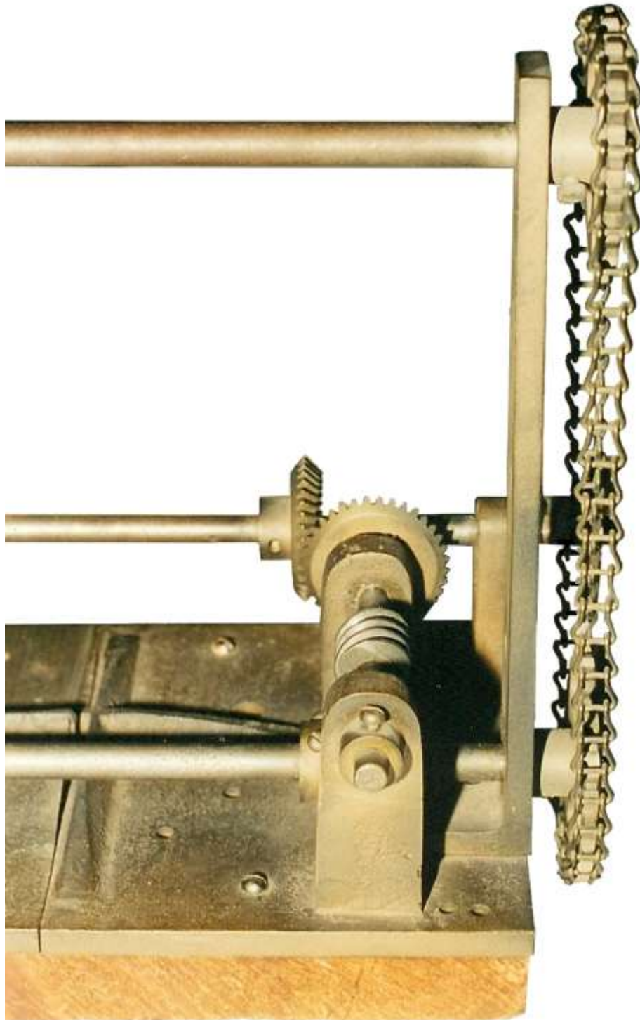
Vitascope projector with a Beater movement Collection George Eastman House, Technology Archive Photo Carey Williams, previously unpublished
