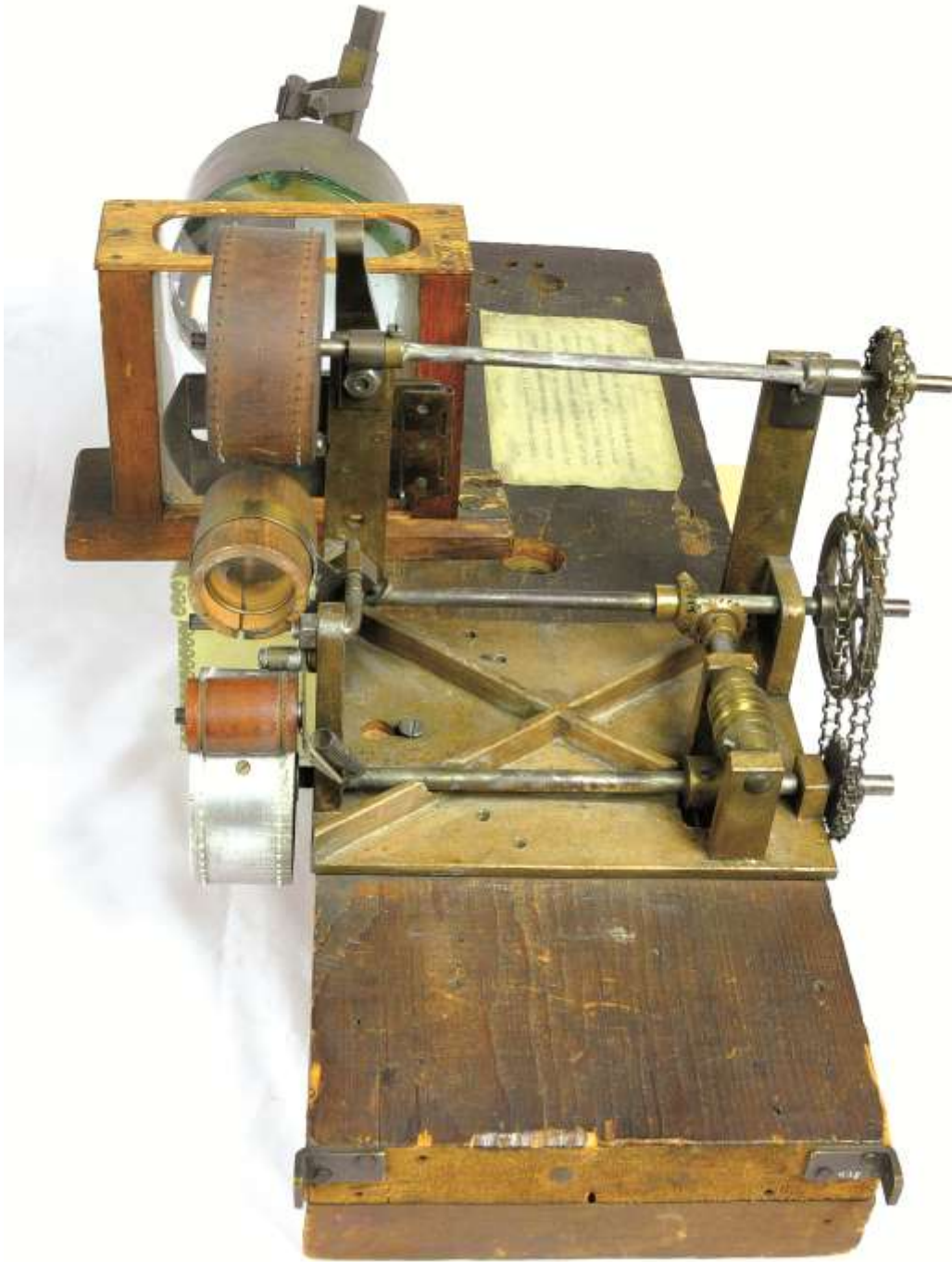
The original Jenkins Phantoscope lateral projector 1893-1894 From the Historical and Interpretive Collections of the Franklin Institute, Philadelphia, PA., photographed at the request of the Author.
