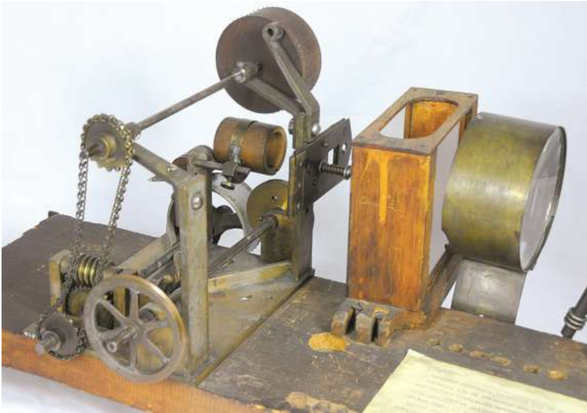
The original Jenkins Phantoscope lateral projector 1893-1894 From the Historical and Interpretive Collections of the Franklin Institute, Philadelphia, PA., photographed at the request of the Author.
