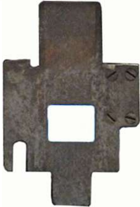
Above Bracket for mounting film gate , below new film gate, added to the Spoolbank Kinetoscope No. 10 Soterios Gardiakos collection
