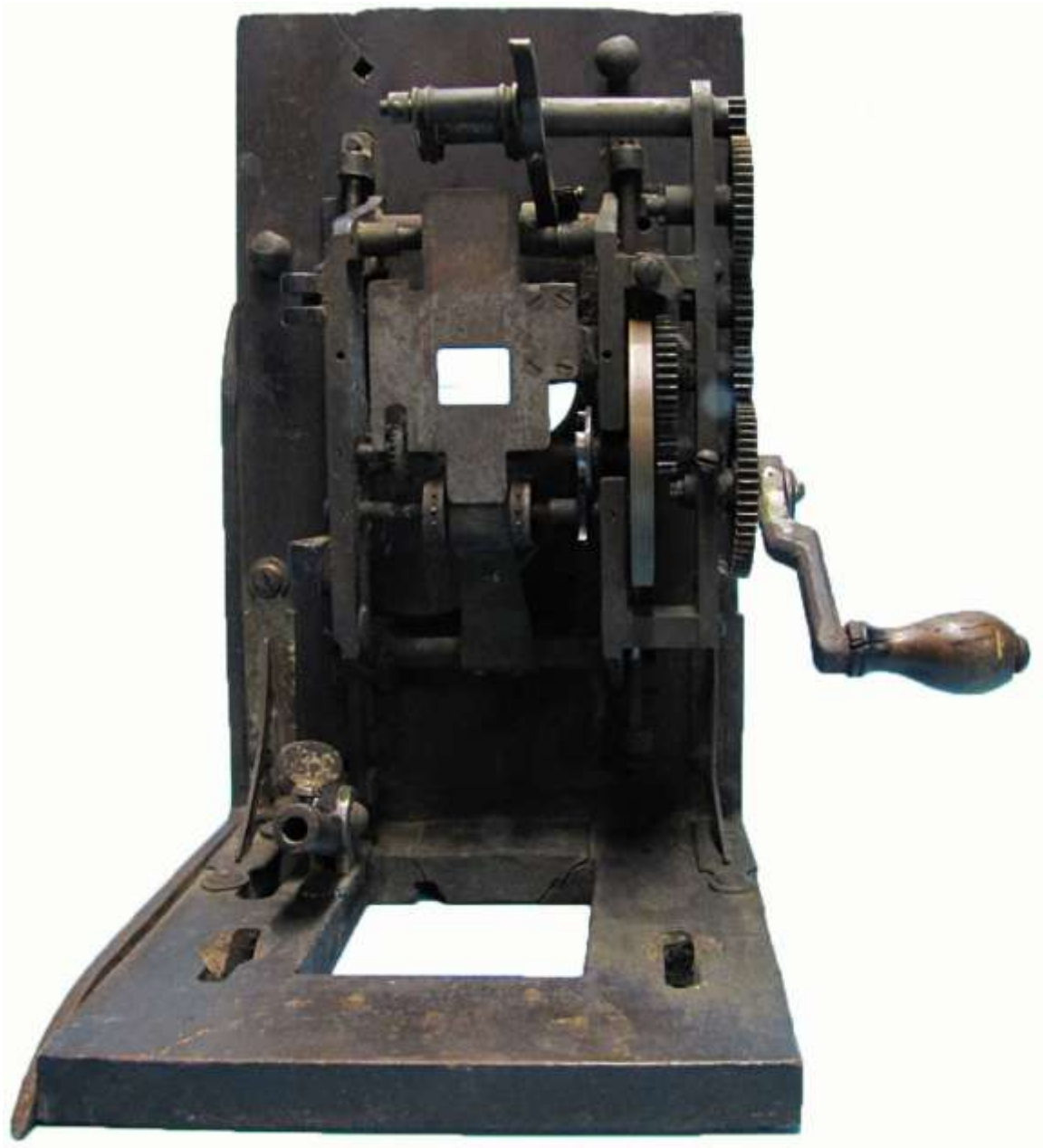
Possibly a later version of Cameragraph No. 1, the chain drive has been replaced with a gear drive Soterios Gardiakos collection
