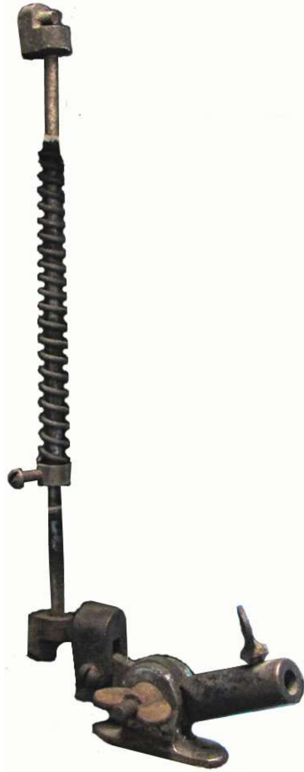
New framer mechanism added to the Spoolbank Kinetoscope No. 10 Soterios Gardiakos collection
